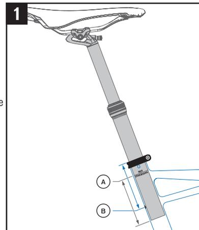
If the seatpost is at the min/max mark and the seatpost does not meet or exceed the minimum measured insertion depth of the frame, the seatpost is not inserted deeply enough into the seat tube and should be lowered until it meets or exceeds the frame insertion requirement. This may result in the saddle being too low. If so, the seatpost must be replaced with a longer seatpost.
